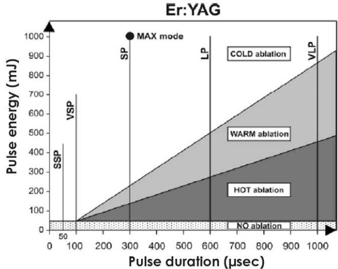
Fig.4: Cold and hot regimes for Fidelis Er:YAG lasers. Nominal pulse durations that apply to situations at high laser energies are depicted for different mode durations.
