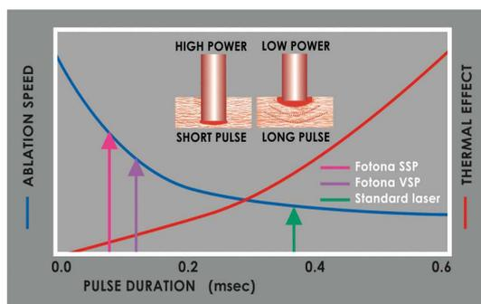
*Fig.6: Keeping the pulse energy constant, the ablation efficiency increases, and the thermal effects decrease towards shorter pulse durations. Due to the long cross-relaxation time of the  $\text{Cr}^{3+}$  ion, the Er,Cr:YSGG cannot be operated below approximately  $500\mu\text{s}$ .*
