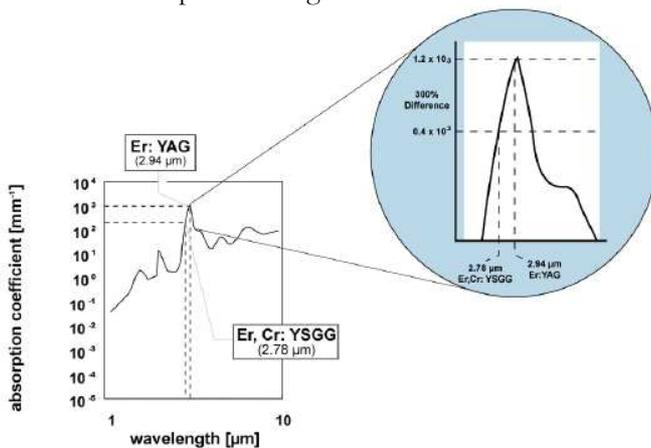
Fig.1: The Er:YAG (2.94  $\mu\text{m}$ ) laser has the highest absorption in water and hydroxyapatite. An alternative laser that emits in the 3  $\mu\text{m}$  region is the Er,Cr:YSGG (2.78  $\mu\text{m}$ ) laser, however this laser has a 300% lower absorption and is thus less suitable for laser drilling.
