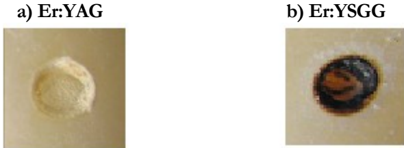
Fig. 9: Pictures of cavities in dentin, made with Er:YAG and Er,Cr:YSGG lasers following three consecutive laser pulses of the same laser pulse fluence of 80 J/cm 2 [19]. In order to eliminate any influence of the difference in pulse duration, the Er:YAG pulse duration (Fotona dental laser, VSP mode) was adjusted to match that of the Er,Cr:YSGG (Waterlase PFN S mode). In this experiment, no water spray was used.
