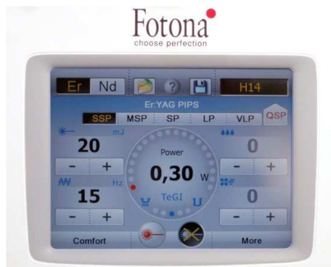
Fig. 5: Touch screen panel showing the PIPSTM setting, at 20 mJ, 15 Hz, no air / no water, 50 microsecond pulse duration.
